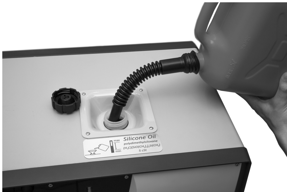
Fig. 17 Filling an oil to cooling unit using special hose.
